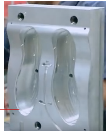
Fig 5.16 CNC milling carves billet creating a positive and negative mould (20 hrs)
