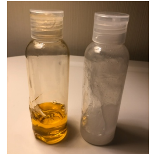
Fig 4.3 Evidence of spill (bottle without prototype)
