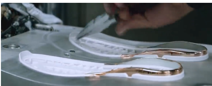
Fig 5.19 Mould must be cured after being pressurised
